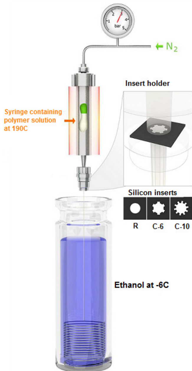
Figure 1. Schematic of fiber extrusion set-up (blow-up shows silicon insert holder and various silicon inserts)
